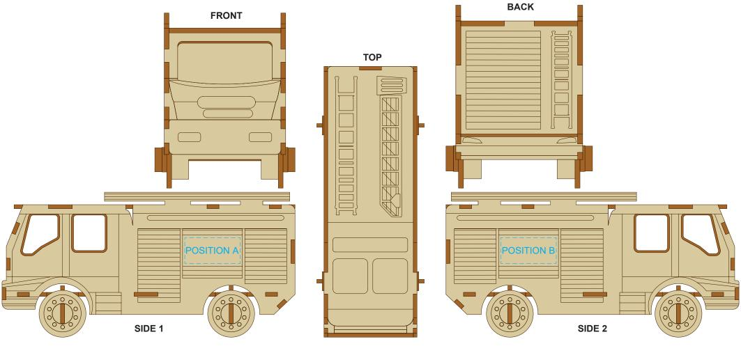
Up to a 2mm tolerance is expected for alignment of the printed artwork against the engraved lines. Slight inconsistencies are to be considered acceptable if the artwork is printed over an engraved line.
